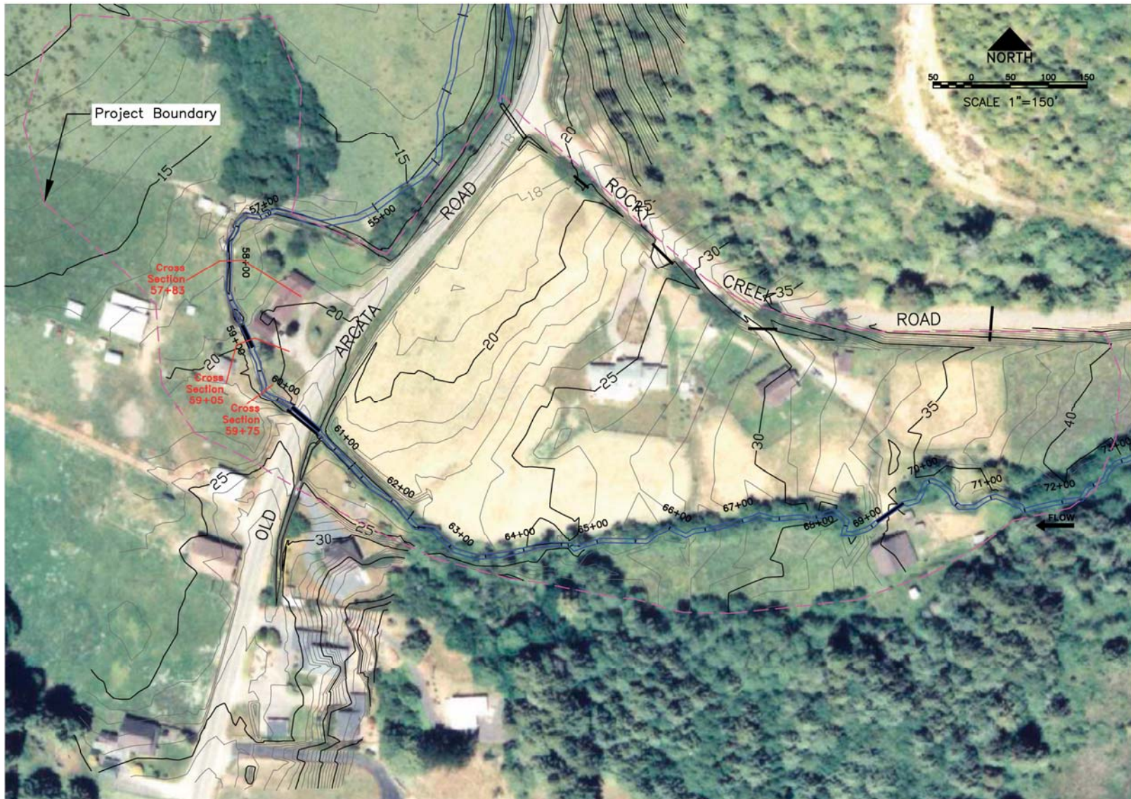
Figure 10. Contour map showing the project boundaries and extent of topographic surveys conducted for the project conceptual design and hydraulic modeling.
